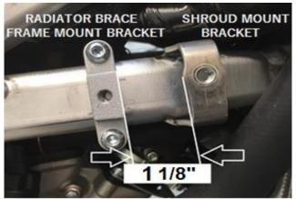
Install the rubber isolator grommet in the 1/2 inch hole of the Radiator Brace. Place the Radiator Brace into position by sliding in under tab as shown.
