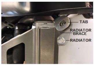
Install the sholdered Allen bolt into the rear hole of the radiator brace and torque to 6 ft./lbs. Install the radiator shroud. Use two of the 6mm x 18mm bolts and washers for the shroud's front upper and lower holes. Install the remaining stock shroud bolts.
